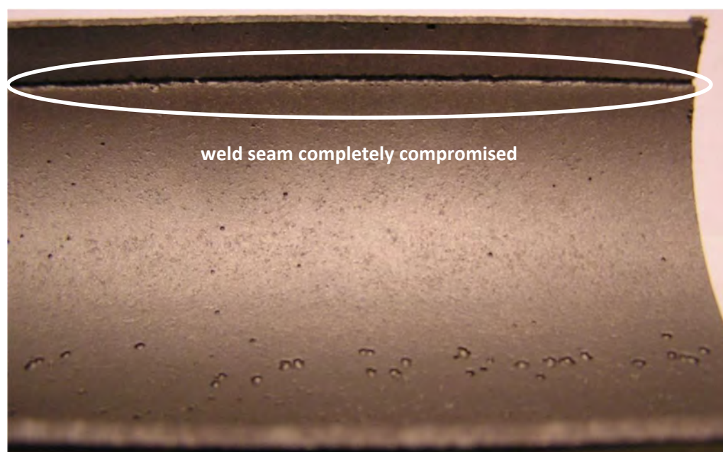
Figure 2: Close-up of weld seam attack by acid corrosion
