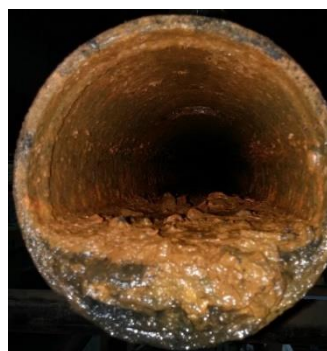
Oxygen Corrosion in Dry Pipe Main
