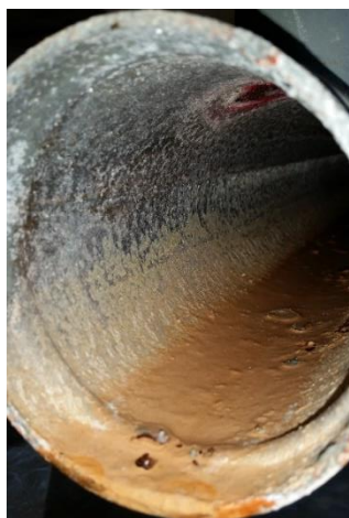
Trapped Water in Galvanized Dry Pipe Main
